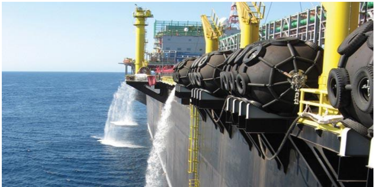
Mariflex.net, FPSO deballasting in action
